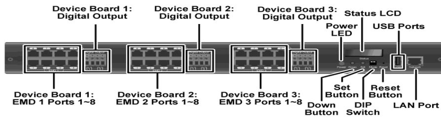
Figure 1-1 interSeptor Pro front view
